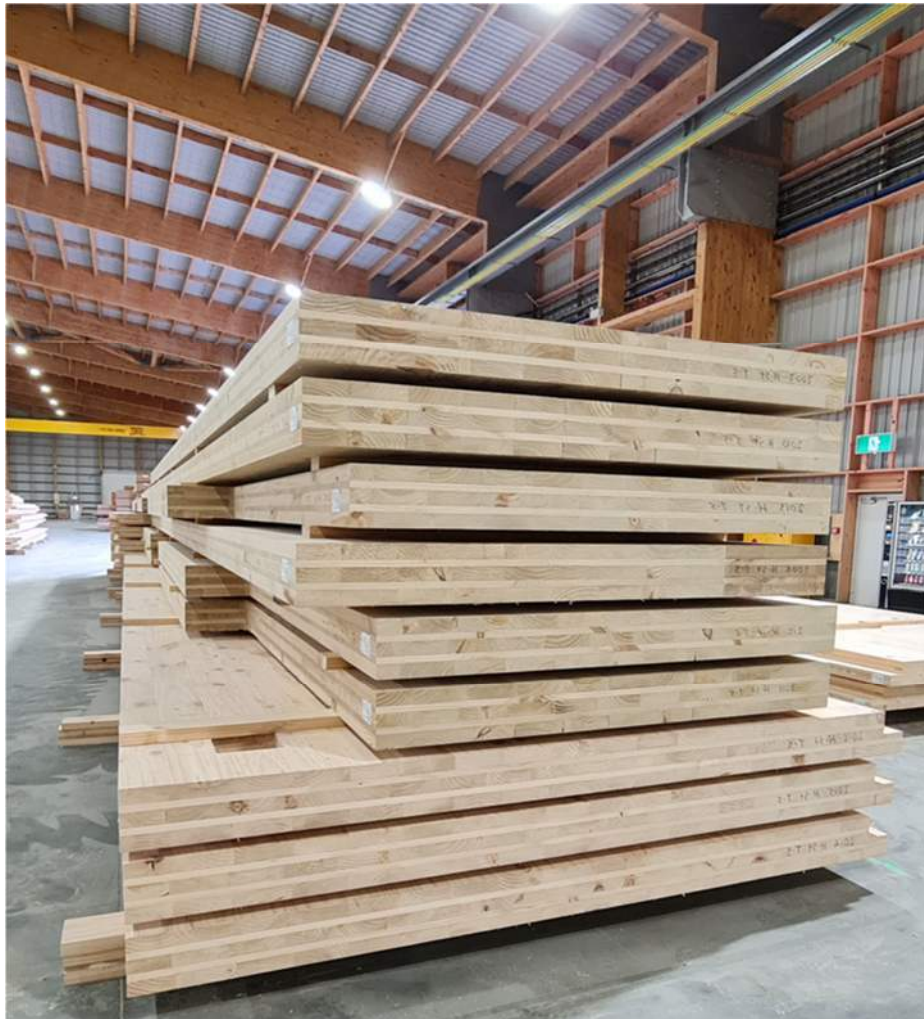
Figure 82: Example of targeted environment and method of storing EWP elements.
