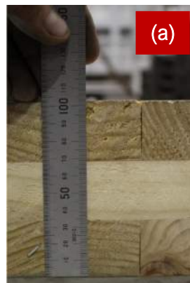
Figure 63: Red Stag CLT system and lamella dimensions.
