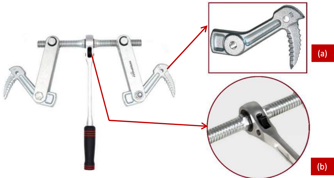
Figure 88: Components of a SKORPIO; a) Hammered in hook at each end; b) Reversible ratchet with sturdy fine thread to allow for fine adjustment [20] .
