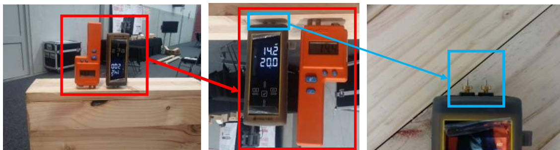
Figure 52: Moisture content measurement of the EWP lamella with suitable timber moisture meters (resistive meters illustrated, but capacitance meters are also acceptable).
