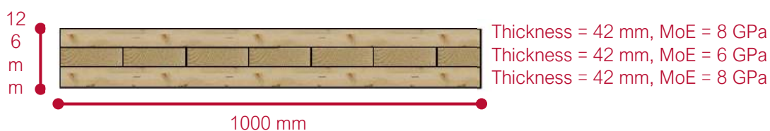
Figure 55: Red Stag CLT Panel Cross-Section.
