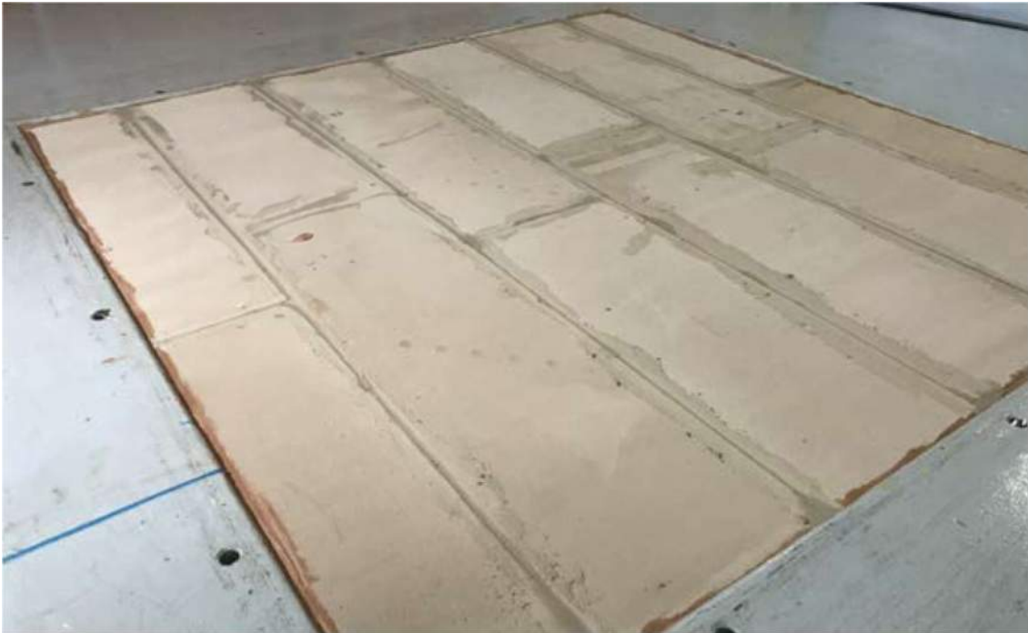
Figure 163: Sample installed in the chamber with tapping machine.
