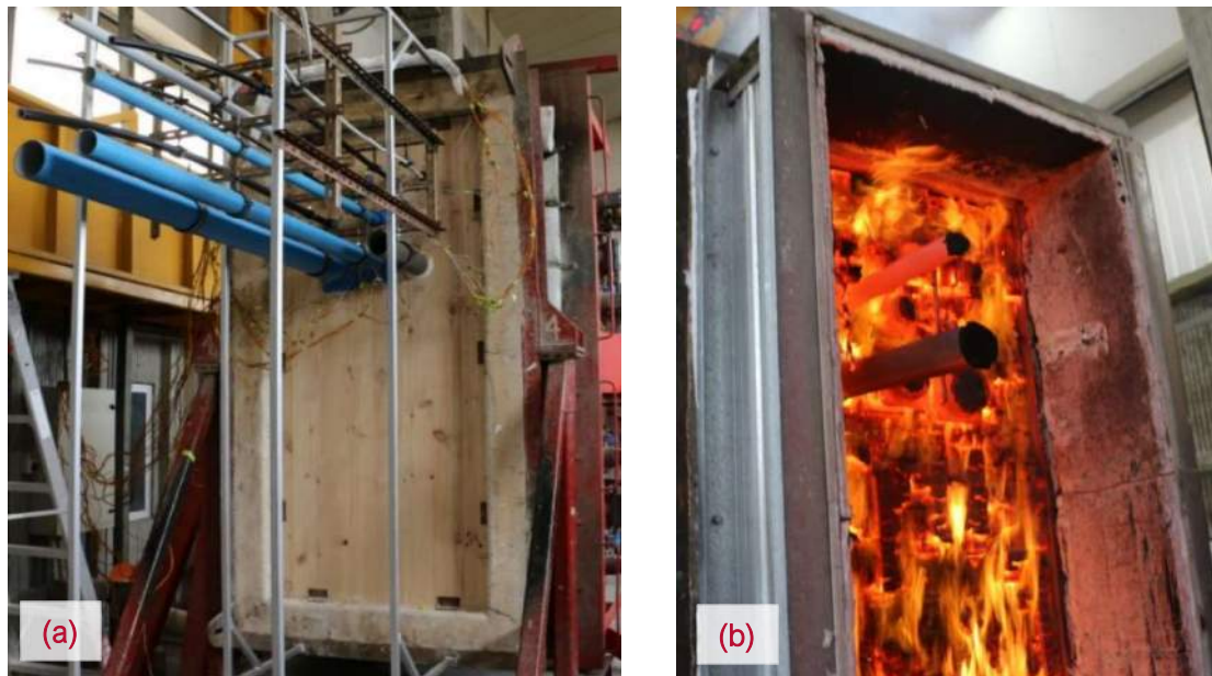
Figure 111: Various service (pipes and cables) fire tests on Red Stag CLT wall panels [26] . a) Specimen before the fire test, b) Specimen after the fire test.
