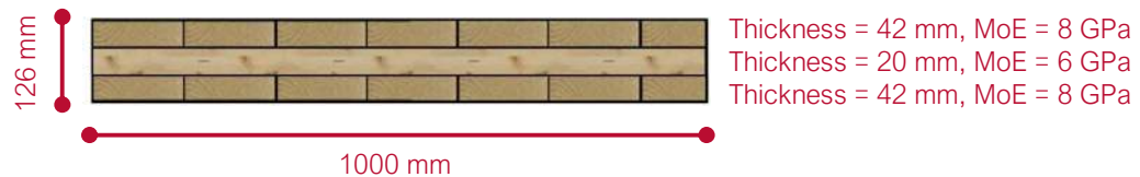
Figure 147: Red Stag CLT Panel Symmetrical Cross-Section
