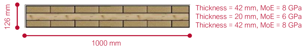
Figure 145: Red Stag CLT Panel Symmetrical Cross-Section
