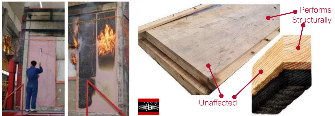
Figure 184: Fire Performance of various timber structural systems; a) Timber frame and truss system, b) CLT composite system without surface protection after 60 minutes fire event.
