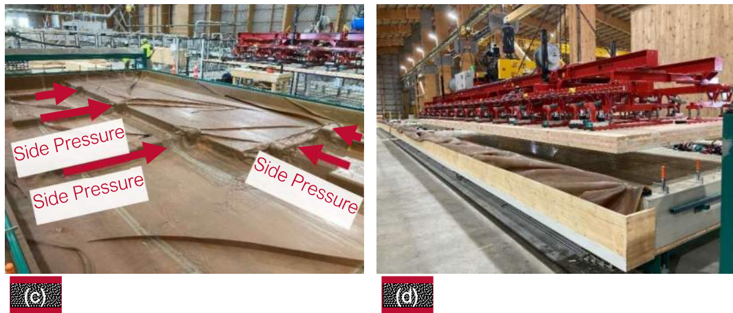
Figure 114: Red Stag Manufacturing line; (a) Layer arrangement with side pressure, (b) Adhesive distribution, (c) Hydraulic side pressure and Vacuum Membrane, (d) Final Red Stag CLT Product.
