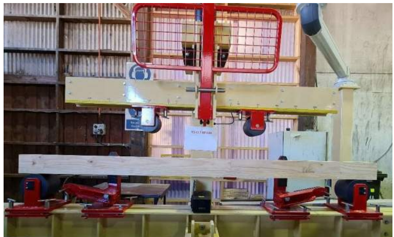
Figure 21: CLT beam bending testing machine and setup; (a) Isometric end elevation; (b) Front elevation.
