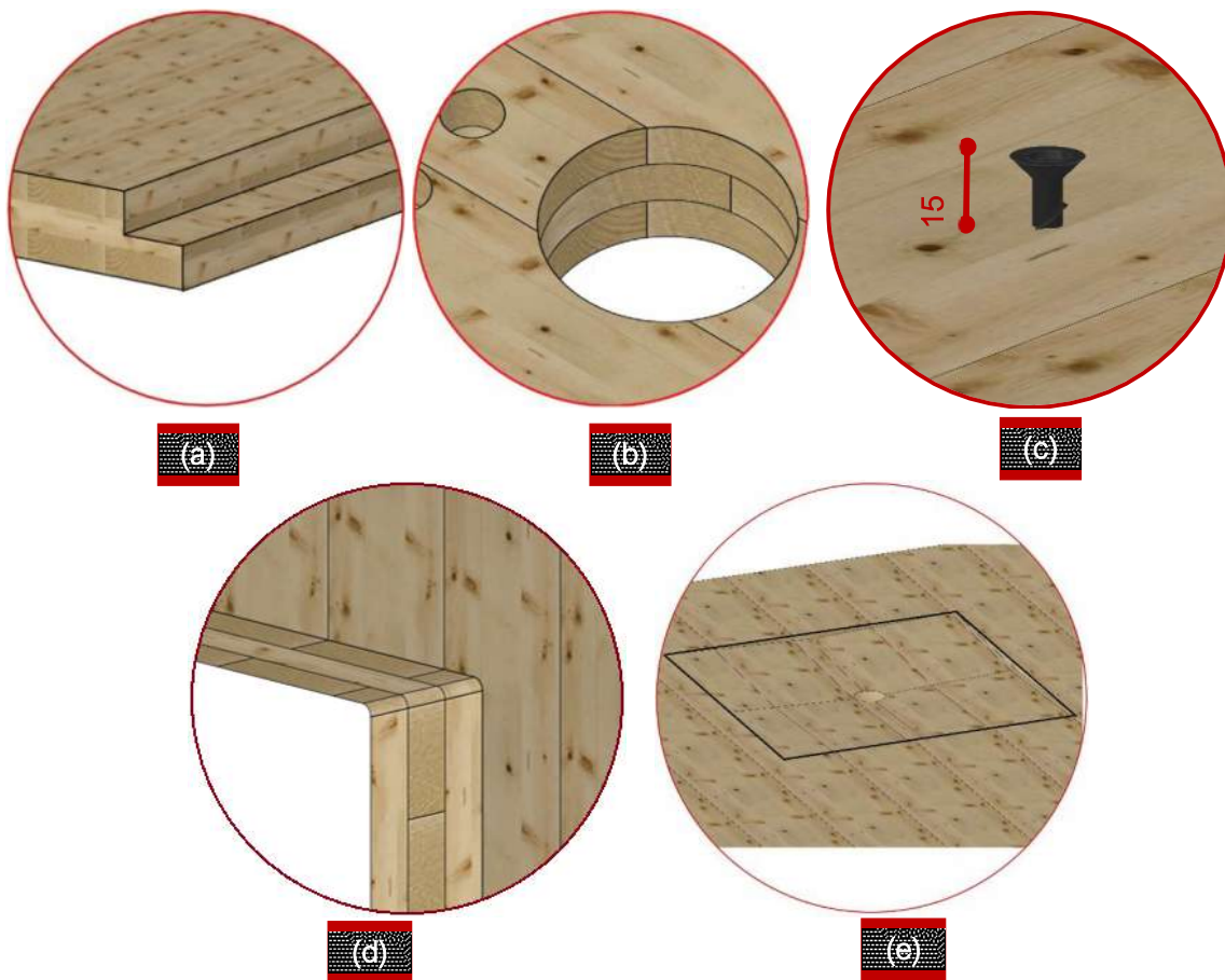
Figure 133: Example of extreme difficulty processing of Red Stag EWP elements; a) Lap/spline joint rebate without flipping or panel removal generally up to 150 mm wide; b) Generally up to eight simple radii penetrations over and above of basic fixing locators; c) Recess for lifting screws; d) Generally up to six openings or two recesses (e.g. doors, windows, trenching) with radii corners or four with square corners subject to tooling restrictions.
