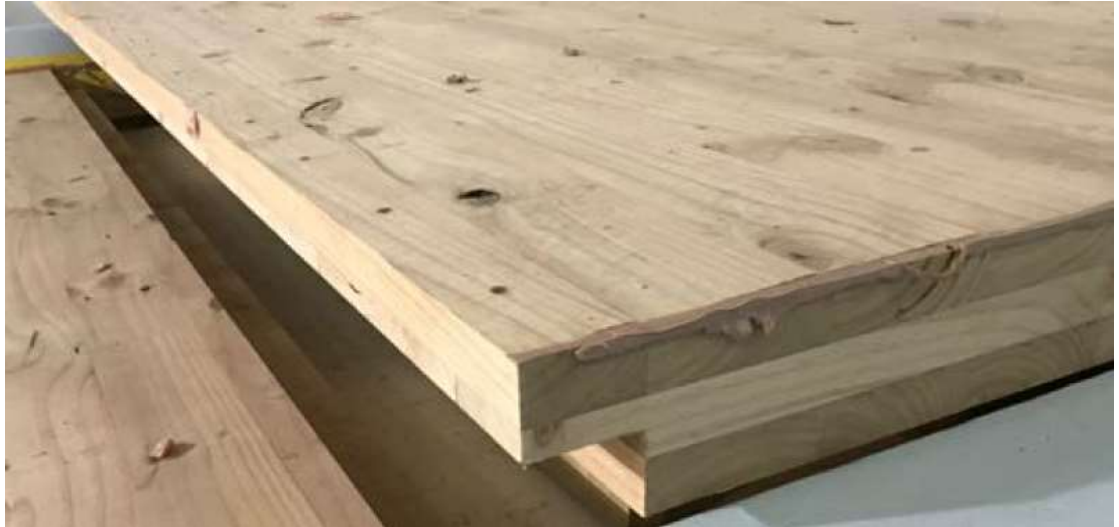
Figure 156: Three-layer Red Stag CLT panel with lap joint.
