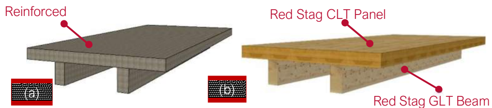
Figure 185: Composite beams; a) Reinforced concrete composite beam, b) Red Stag CLT composite beam.
