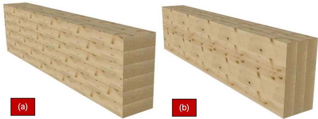
Figure 169: GLT 3D views; a) GLT horizontal brick layout; b) GLT vertical brick layout.
