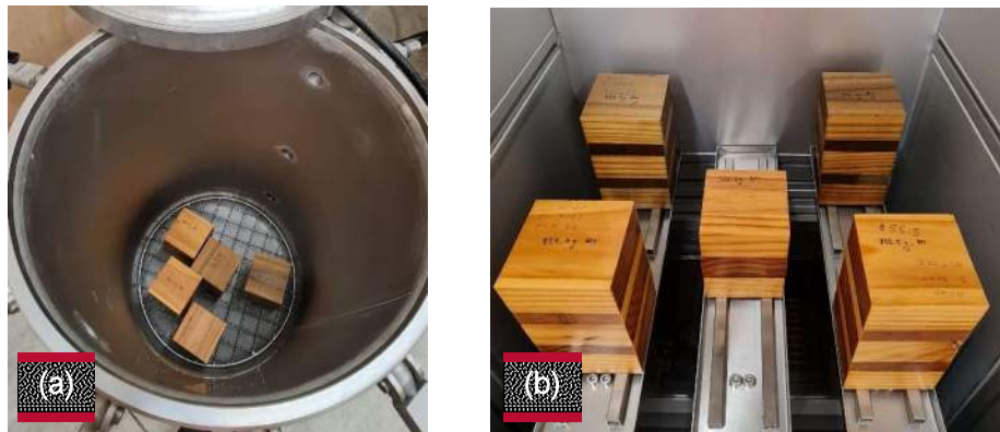
Figure 126: Delamination testing equipment; a) EWP specimens in pressure vessel; b) EWP specimens in drying chamber.
