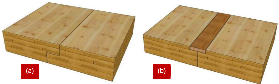
Figure 34: CLT floor to CLT floor panel connection; a) Lap joint; b) Spline joint.
