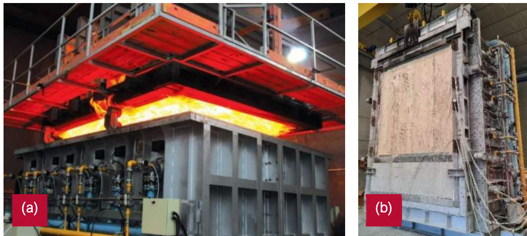
Figure 127: Large-scale fire testing on Red Stag EWP conducted by BRANZ; (a) Red Stag CLT floor test specimen after fire testing; (b) Red Stag CLT wall test specimen before fire testing.
