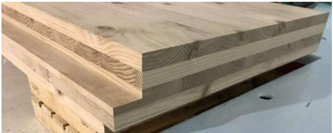
Figure 157: Five-layer Red Stag CLT panel with lap joint.
