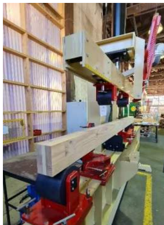
Figure 21: CLT beam bending testing machine and setup; (a) Isometric end elevation; (b) Front elevation.
