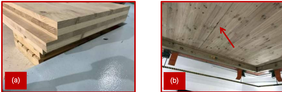
Figure 155: 210 mm thick five-layer Red Stag CLT panel with lap joint installed in the acoustic chamber at the testing laboratory.
