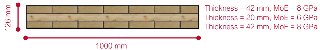
Figure 150: Red Stag CLT Panel Symmetrical Cross-Section
