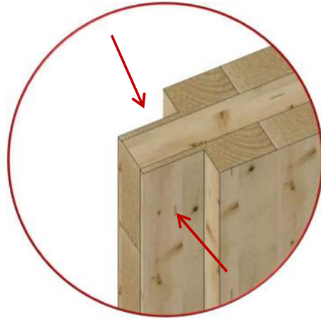
Figure 134: Double Spline Joint Plate Connection with two sides CNC process.
