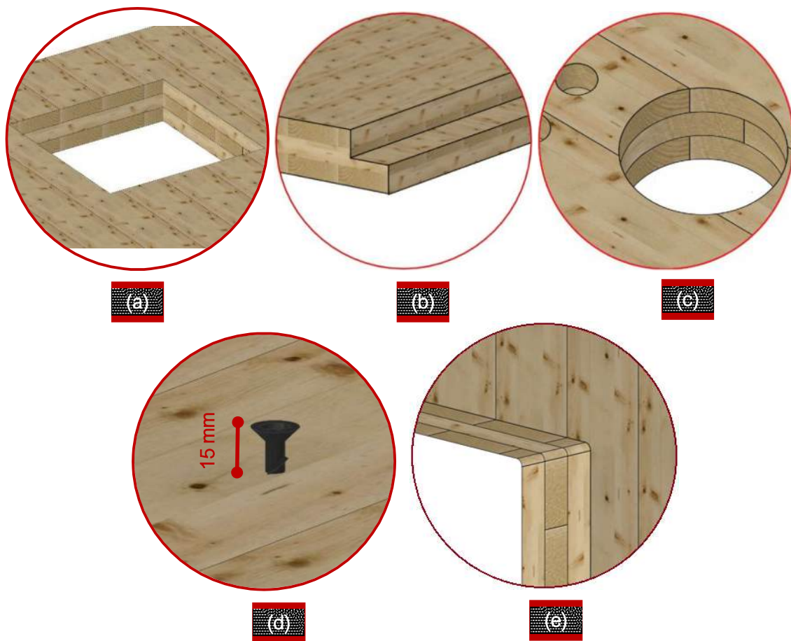
Figure 132: Example of very difficult complexity processing of Red Stag EWP elements; a) Up to three square cut outs (subject to minimum size for tooling); b) Lap/spline joint rebate without flipping or panel removal up to 120 mm wide; c) Up to six simple radii penetrations over and above of basic fixing locators; d) Predrilling/installation of lifting screws; e) Door or window corner on Red Stag CLT Wall Panel (either four radii openings or three-square openings).
