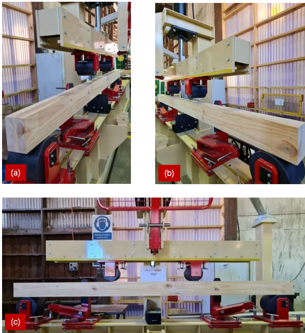
Figure 191: Large-scale mechanical testing of Red Stag CLT beams conducted by Red Stag; a & b) End Elevation; c) Elevation.
