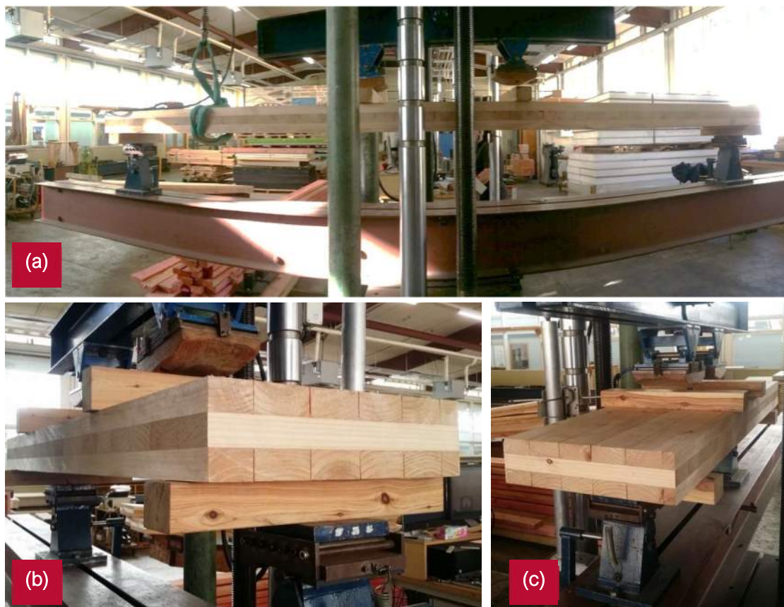
Figure 125: Large scale mechanical testing conducted by SCION; (a) Long span testing; (b) Medium span testing; (c) Short span testing.
