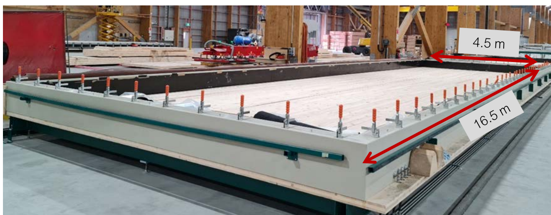
Figure 2: One of Red Stag's CLT vacuum presses.
