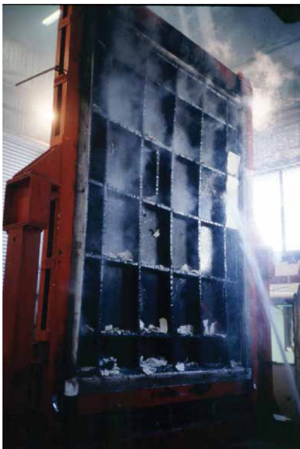
Full scale fire resistance test of a light timber framed wall. Credit BRANZ.
