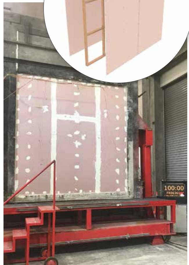
Full-scale fire resistance test of a light timber framed wall. Credit BRANZ.
