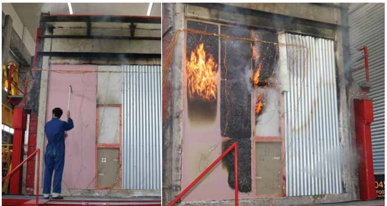
Fire testing of light timber framed walls at BRANZ. Credit BRANZ.
