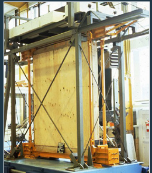
Light timber frame shear wall being tested.
