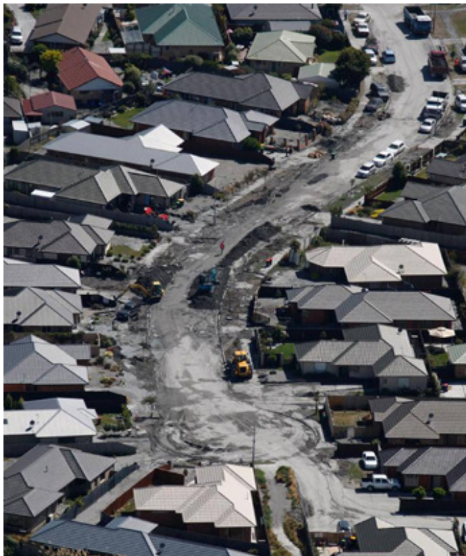
Damage following the 2011 Christchurch earthquake showing the extensive liquefaction that impacted residential housing.
