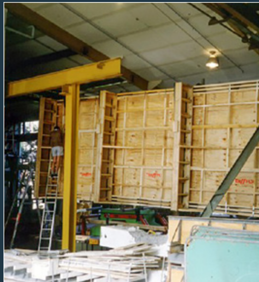
Lateral load testing of a three-storey light timber frame shear wall.
