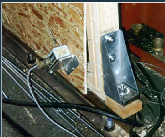
Hold down and wall toe performance of a light timber frame shear wall.
