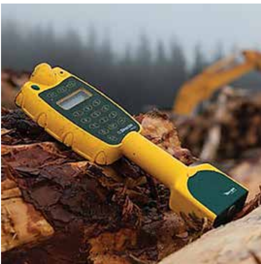
Figure 9. Use of an impact (sonic) device to sort logs.
