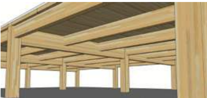
Two-way Beam System.
