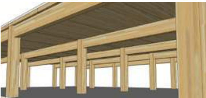
One-way Beam System.
